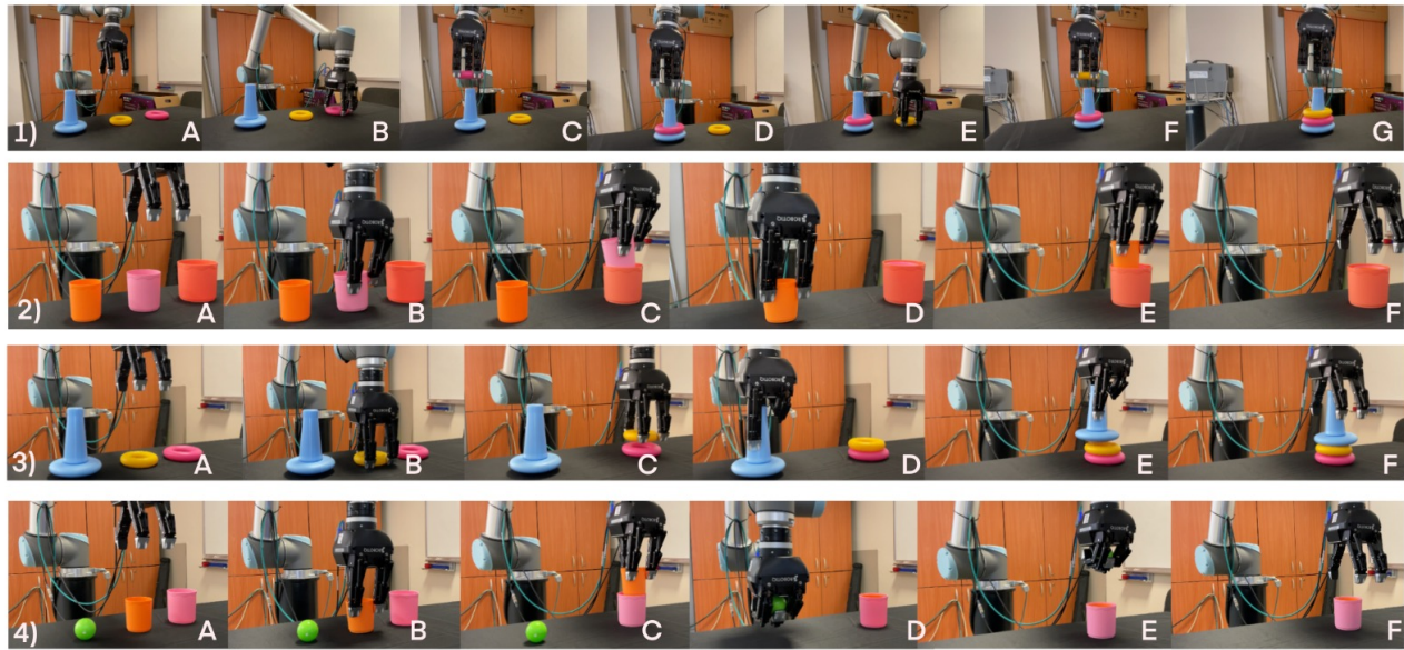
Fig. 7. A number of snapshots from real-world planning experiments. In the first, second, and fourth images, the objective is to construct the shortest compound objects. In the third image, the goal is to create the tallest compound object. The system observes the scene, predicts the effects of each potential plan using MOGAN, and executes the optimal one.
