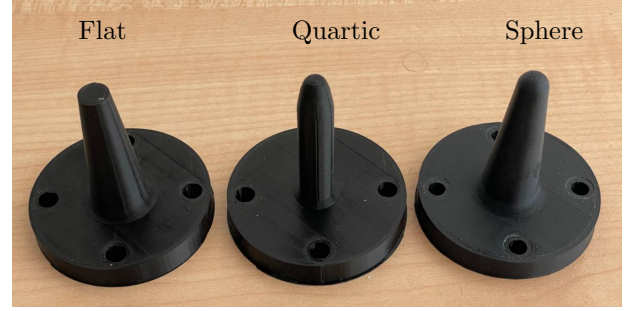
Fig. 6. 3D-printed tips utilised in the experiments. From left: the flat, the quartic and the spherical tips.
