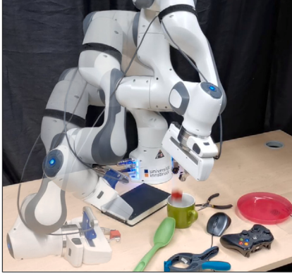
Fig. 1. Our work combines off-the-shelf deep learning strategies to detect objects in the clutter, and imitation learning to realize complicated trajectories, e.g., dropping a cube into a cup on an untidy table. The large projection formulation combines the two machine learning components and ensures convergence to a given target.
