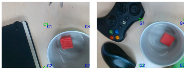
Fig. 14. Two final image frames captured by the robot camera showing that IL-DVS successfully drives the robot to drop the object into the cup in different cluttered environments.
