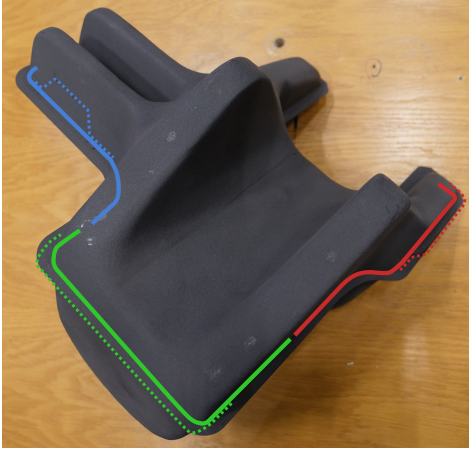
Fig. 7: Approximate positions of test path 1 (red), test path 2 (green), and test path 3 (blue) and their respective corrections (dotted lines) on the test object.
