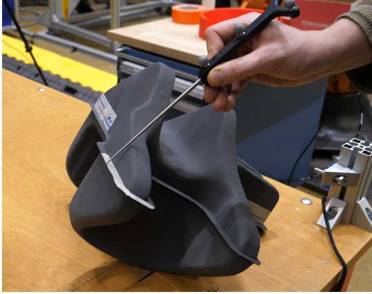
Fig. 4: Test object and tracking tool (NDI Polaris Vega XT) used for path model teaching and path demonstrations.
